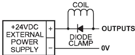
**Note:** For inductive loads, customers must connect a clamping diode to protect from flyback voltage spikes.
